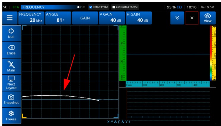
Figure 4-46 Lift Off Signal
