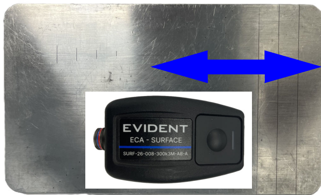
Figure 4-8 Adjusting the Defect Amplitude
