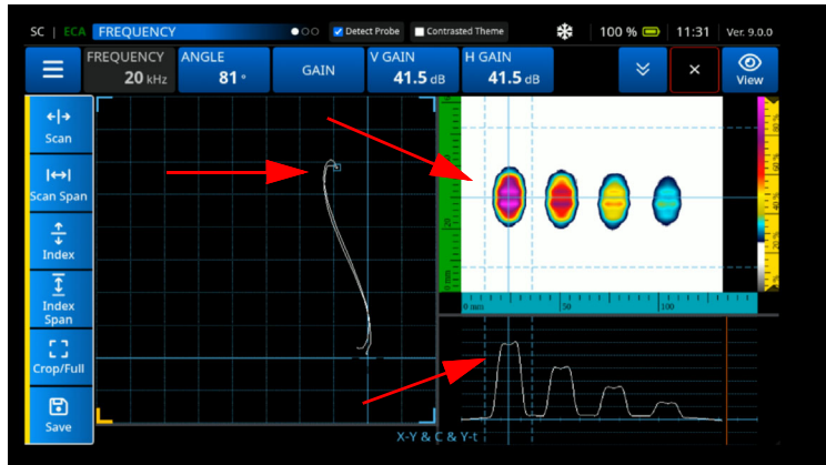
Figure 4-51 Select Deepest Corrosion Spot
