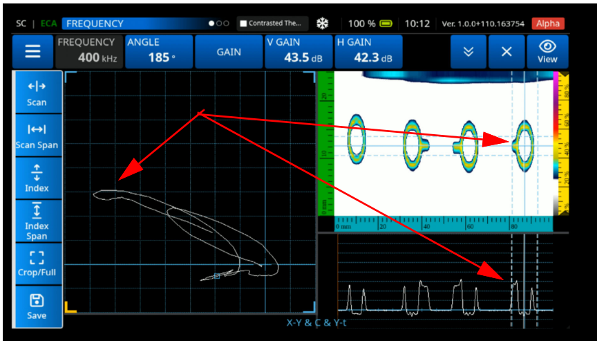
Figure 4-90 Set V Gain for Cracked Fastener
