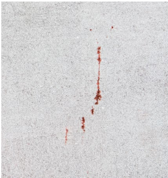
Red dye penetrant indications
